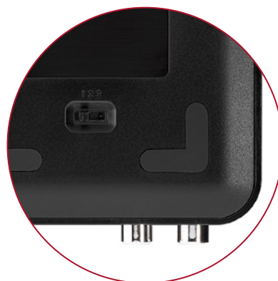
A switch on the underside of each JLINK™ unit assigns it to one of three RF channels, allowing multiple JLINK™ systems to operate independently in a home.
