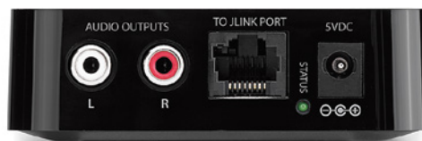
The JLINK™ Receiver offers analog outputs via RCA-type jacks or a direct, powered connection to the JLINK™ port on a compatible JL Audio subwoofer.
